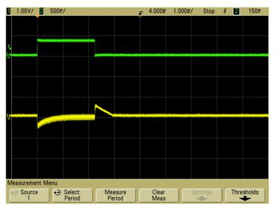
Figure 4: Transient response of a stabilized switching regulator
